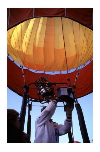
4 The bottom of a hot air balloon is open. A burner below the opening heats the air inside the balloon. Hot air fills the balloon and the balloon rises.
