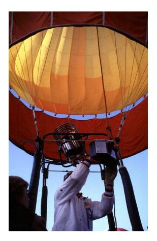
4 The bottom of a hot air balloon is open. A burner below the opening heats the air inside the balloon. Hot air fills the balloon and the balloon rises.
