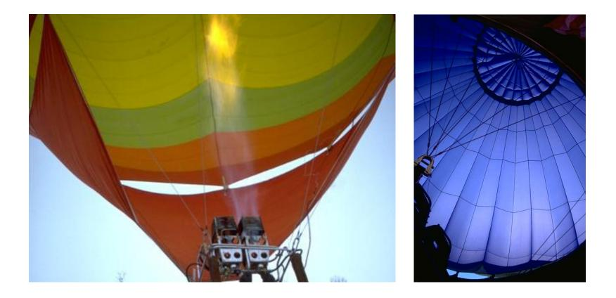
To make the balloon rise, the pilot turns the burner up. The flames heat the air. To make the balloon go lower, the pilot turns the burner down so the air cools.
